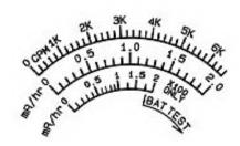
Most survey meters have scales that read in milliRoentgen per hour (mR/hr) and/or counts per minute (cpm) or counts per second (cps). After detector efficiency is taken into consideration, the cpm or cps scales give an indication of the quantity of radioactivity. The mR/hr scales give an indication of the radiation exposure rate. There is an important difference in these measurements. Exposure rate measurements are only valid for electromagnetic  $(x-/\gamma)$  radiation.
