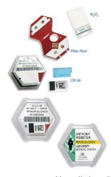
Auburn University currently uses optically stimulated luminescence (OSL) dosimeters and thermoluminescent dosimeters (TLDs) supplied and processed by an independent outside company. Other types of dosimeters such as film badges may also be used.
