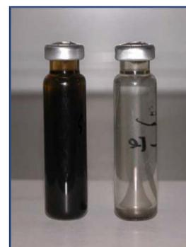
Visual comparison of nano-particle stability after five days: stabilized (left) vs. unstabilized (right)
