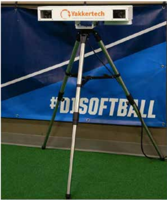
Figure 1. Yakkertek Device Used to Measure Batted Ball Characteristics
