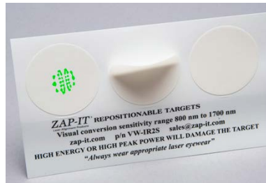
Figure 4: ZAP-IT Laser Alignment Paper
