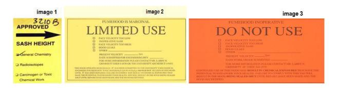
In general chemical fume hood sash heights shall maintain at 18 inches or less unless otherwise specified by the chemical fume hood manufacturer.
