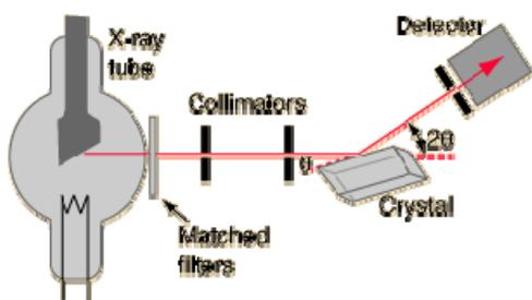
X-ray diffraction wavelengths ( $\lambda$ ) are selected so as to roughly correspond to the inter-atomic distances within the sample, and to minimize fluorescence. Wavelengths commonly used are 1.54 Å (Cu targets), 0.71 Å (Mo targets), 0.56 Å (Ag targets), and 2.3 Å (Cr targets). The relationship between wavelength and x-ray photon energy is determined by the equation
