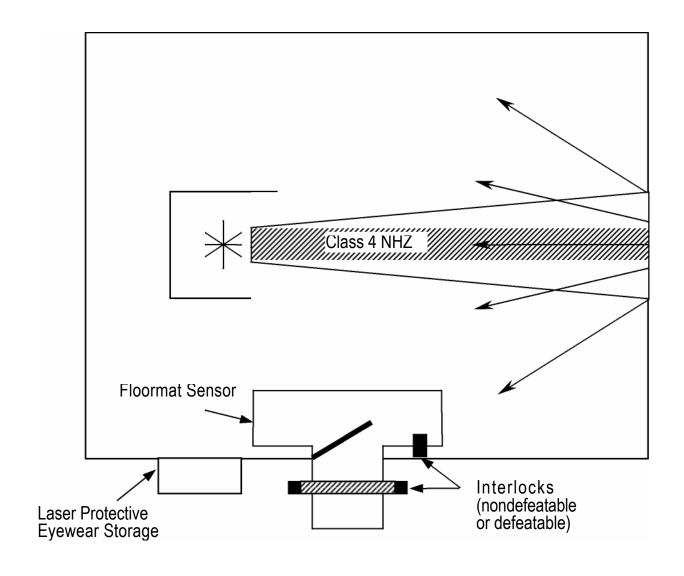
Figure 2a. Area/Entryway Safety Controls for Class 4 Lasers Utilizing Entryway Interlocks
