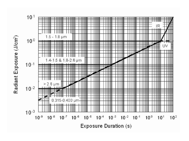
Figure 6. MPE for Ultraviolet (Wavelengths from 0.315 to 0.400 m) and Infrared Radiation (Wavelengths from 1.400 m to 1mm) for Single Pulses or Continuous Exposure (Small or Extended Sources)
