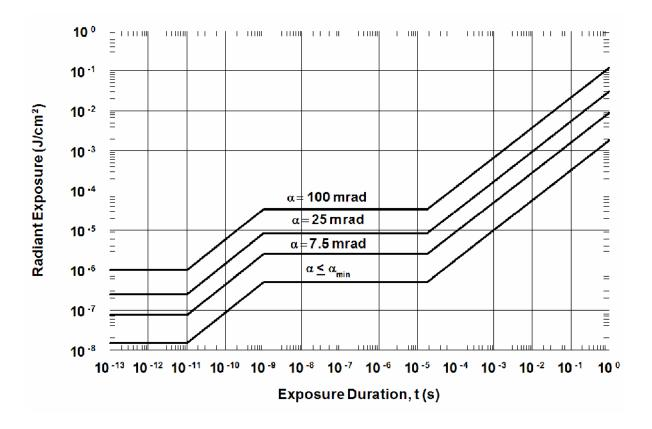
Figure 7. MPE for Ocular Exposure to Visible Laser Radiation (Wavelengths from 0.400 to 0.700 m) for Single Pulses or Continuous Exposure (Small or Extended Sources)
