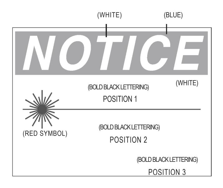
Figure 1d. Sample Warning Sign for Facility Policy, for example, Outside a Temporary Laser Controlled Area During Periods of Service
