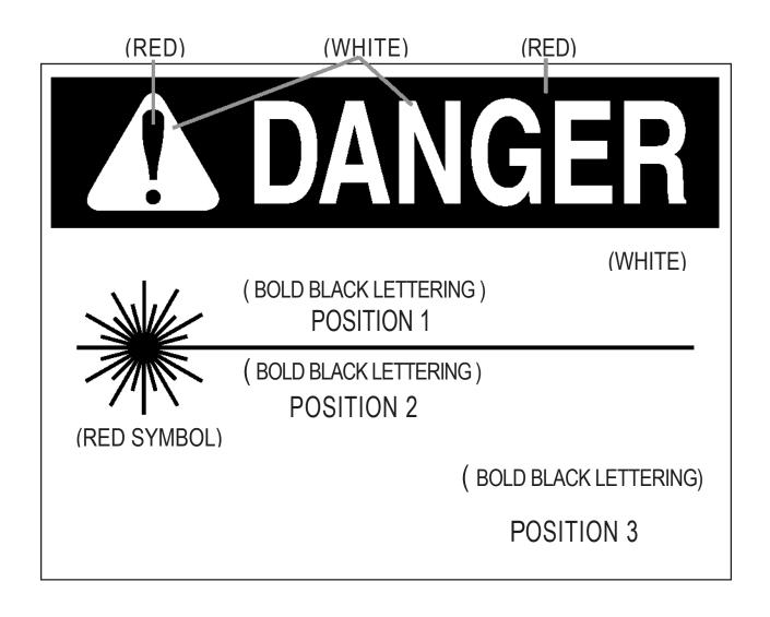
Figure 1b. Sample Warning Sign for Class 3R, Class 3B, and Class 4 Lasers
