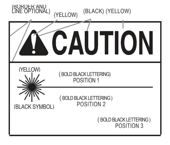
Figure 1a. Sample Warning Sign for Class 2 and Class 2M Lasers
