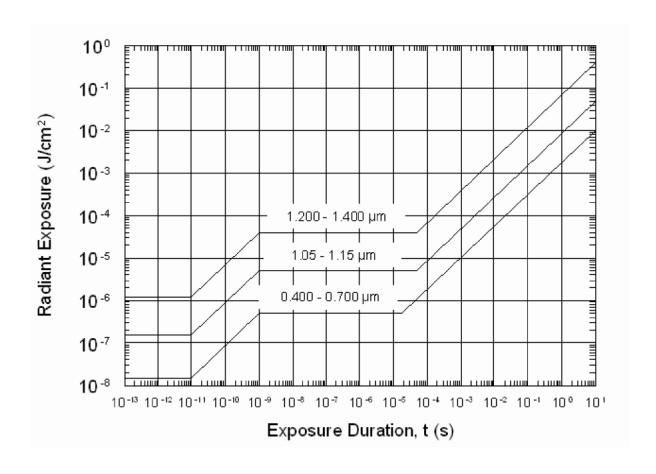
Figure 4. Point Source MPEs for Visible and Near Infrared Pulsed Sources (Wavelengths from 0.400 to 1.400 m)
