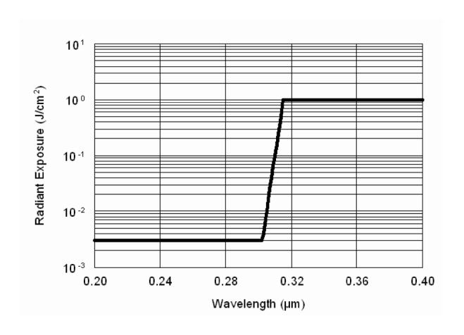
Figure 5. MPE for Ultraviolet Radiation (Small and Extended Sources) for Exposure Duration from  $10^{-9}$  to  $3\ 10^4$  s for Ocular Exposure and  $10^{-9}$  to  $10^3$  s for Skin Exposure\*
